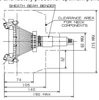
Fig. 8 – Neck Component Detail
