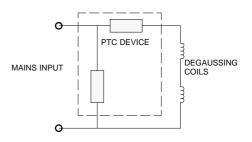
Fig. 11 - Typical Degaussing Circuit
