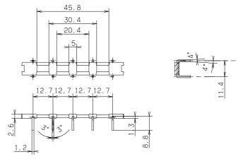
Fig. 2 - Yoke Terminal Board
