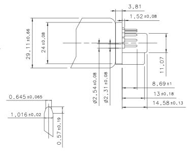
Fig. 7 - Pin Connections and Rear view of Base
