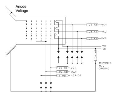
Fig. 12 – Picture Tube Connections Showing Spark–Gaps Recommendations and Typical Isolation–Resistor Values.
