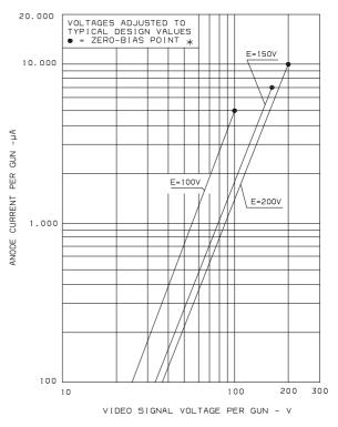
\* Under normal operating conditions, the cathode voltages should not go within 10 volts relative to the grid-no. 1.
