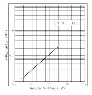
Fig. 3 – X–Radiation Limit Curves at a Constant Anode Current of 300  $\,\mu\text{A}$  (X–radiation at a constant anode voltage varies linearly with anode current)
