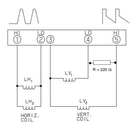
Fig. 1 – Connection Diagram Bottom Board
