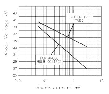
Fig. 9-0.5 mR/h Isoexposure-Rate Limit Curves
