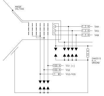
\* If a G<sub>1</sub> bias voltage source is used, the isolation resistor and spark gap is required. Direct grounding of the G<sub>1</sub> to the low voltage spark gap ground at the tube socket is permissible. In this case, a G<sub>1</sub> spark gap is not required.
