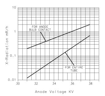
Fig. 9 - X -Radiation Limit Curves at a Constant Anode Current of  $300 \ \mu A$  (x-radiation at a constant anode voltage varies linearly with anode current).
