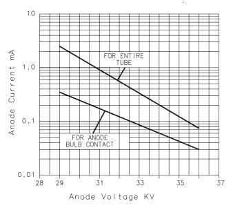
Fig.6 - 1  $\mu$ Sv/h Isoesposure-Rate Limit Curves
